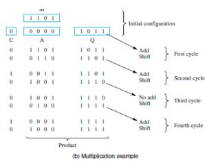
In this, the 4 bit multiplier is stored in Q register, the 4 bit multiplicand is stored in register B and the register A is initially cleared to zero. The multiplication process starts with checking of the least significant bit of B whether it is 0 or 1.
