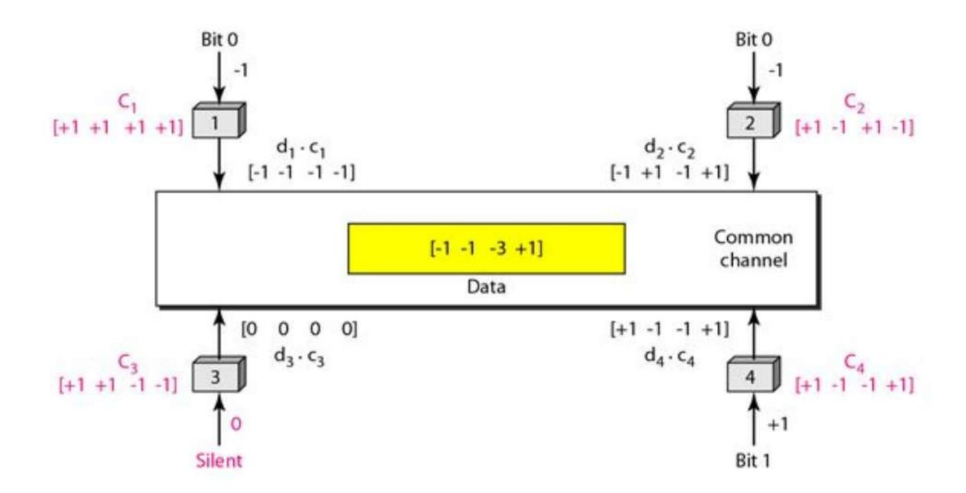
Now imagine station 3, which we said is silents is listening to station 2. Station 3 multiplies the total data on the channel by the code for station 2, which is [+1 -1 +1-1], to get
