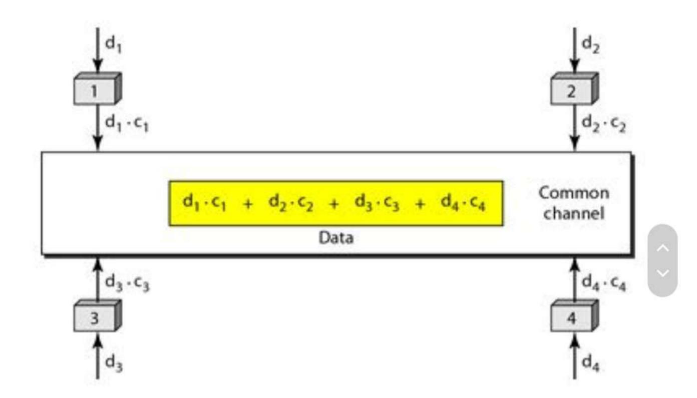
Station 1 multiplies (a special kind of multiplication, as we will see) its data by its code to get d1.c1. Station 2 multiplies its data by its code to get d2.c2. And so on. The data that go on the channel are the sum of all these terms, as shown in the box.
