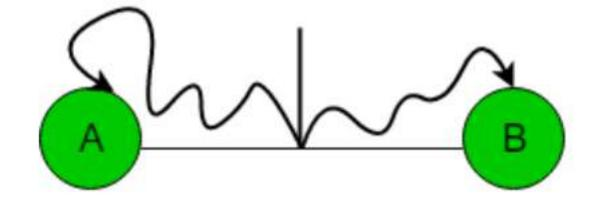
Both stations A and B detect collision
