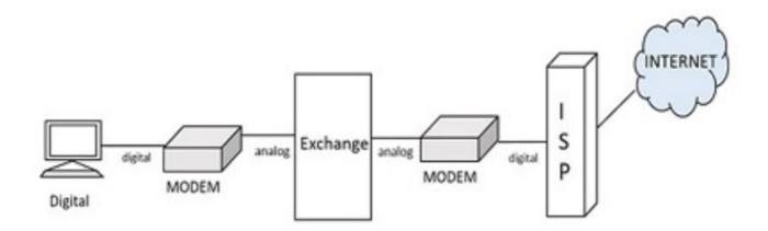
The above figure shows that the digital signals have to be converted into analog and analog signals to digital using modem during the whole path. What if the digital information at one end reaches to the other end in the same mode, without all these connections? It is this basic idea that lead to the development of **ISDN**.
